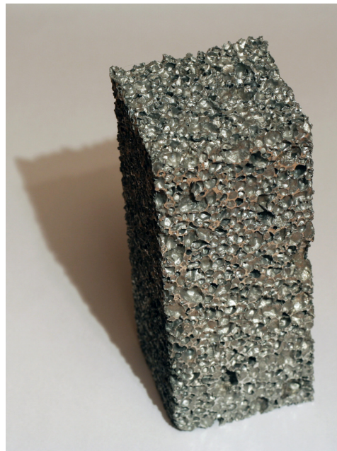
Figure 8. Foamed aluminium, size is around 0.1m. (from Wikipedia)
