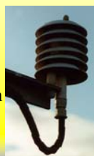
Physics platinum resistance thermometer on Fraser Noble building; photo JSR
