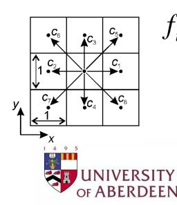
$$f_i^{eq} = w_i \rho \left[ 1 + \frac{u_\alpha c_{i\alpha}}{c_s^2} + \frac{(u_\alpha c_{i\alpha})^2}{2c_s^4} - \frac{u_\alpha u_\alpha}{2c_s^2} \right]$$
