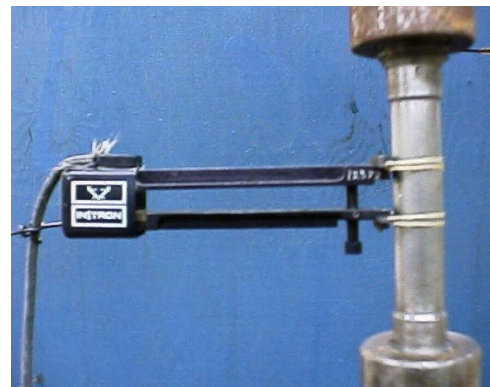
0.1" Range, 0.5" Gage Length Strain Gage Extensometer, Instron Model 2620-826
