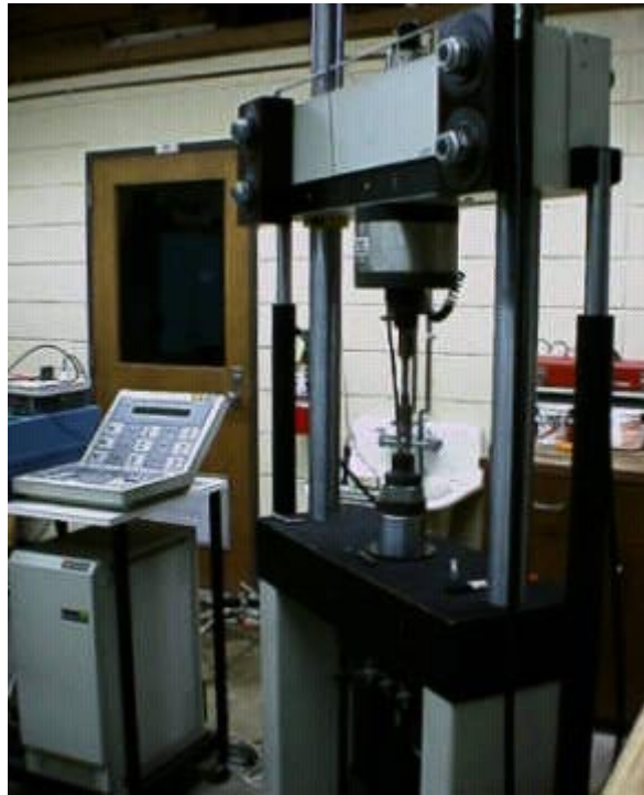
8500 Series Instron Servohydraulic Universal Testing Machine - 50,000 Pound Capacity
